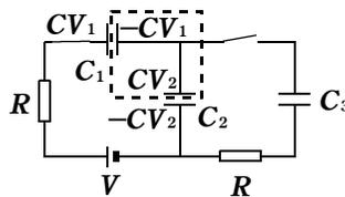
$$-CV_1 + CV_2 = 0 \Leftrightarrow V_1 = V_2$$
