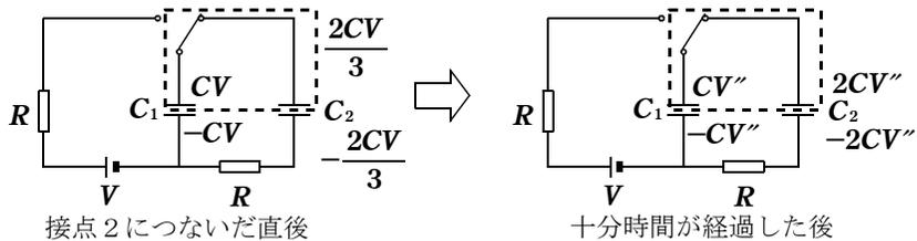
$$CV + \frac{2}{3} CV = CV'' + 2CV'' \Leftrightarrow V'' = \frac{5V}{9}$$
